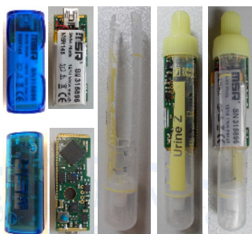
Fig. 2: Mini data logger in protective case, without protective case, empty tube and logger in tube
